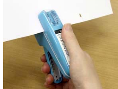
Harinacs: This staple-less stapler works by clipping a small incision into a piece of paper and twisting to form a bond. The papers can later be easily separated again simply by pulling the pages apart.
