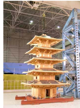
Testing the earthquake resistance of a five-story pagoda. (C)NPO Corporation Forum for Wood Architecture / Building Research Institute
