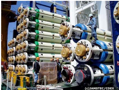
Riser pipes on deck ready for use. (C)Japan Agency for Marine-Earth Science and Technology
