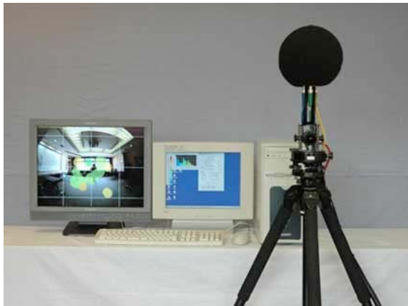
The NoiseCam real-time sound camera. (C)CHUBU Electric Power Co., Inc.
