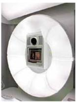
Inside the photo booth is a high-capacity flash lamp and a monitor below the camera for checking the photos.
